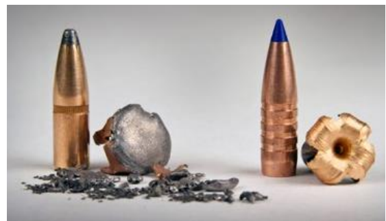
On left: Lead bullet and its fragments after impact. Lead bullets typically lose up to 40 per cent of their mass following impact. On right: A solid copper bullet with a plastic tip. Copper bullets generally lose 0–5% of their mass. Source: huntingwithnonlead.org
